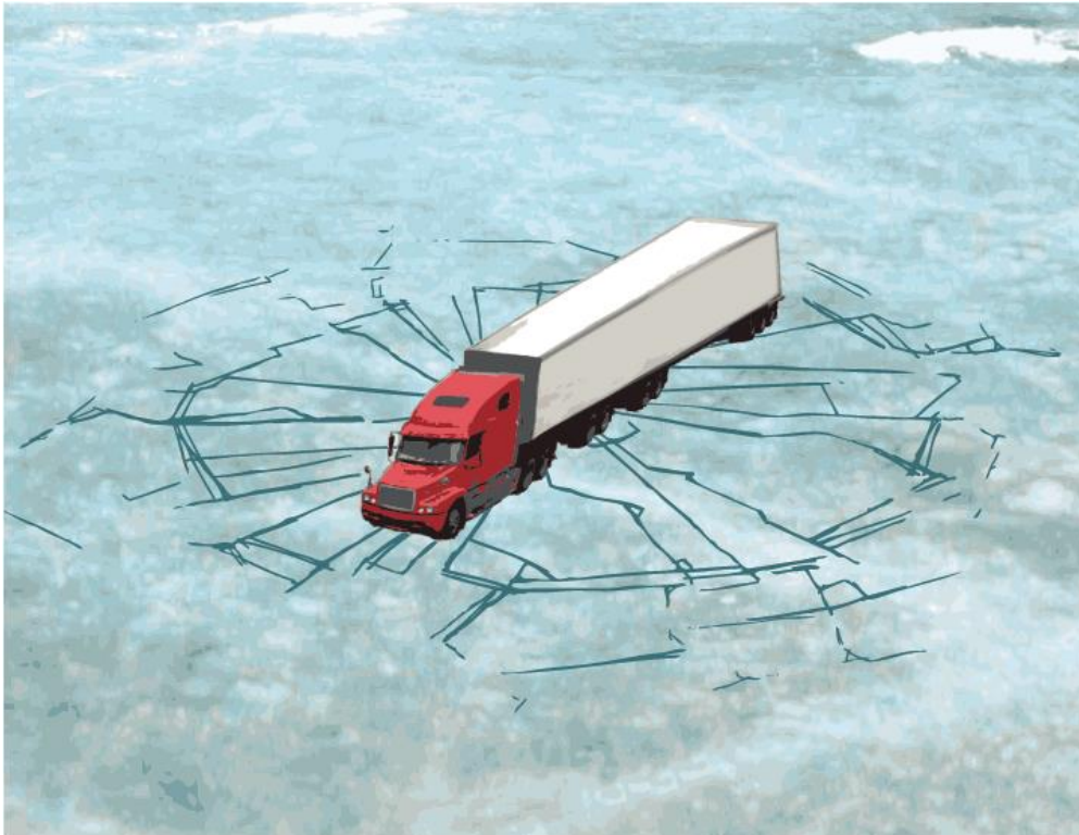
Figure 2 - Aerial View of radial (spoke-like) and circumferential (round) cracks forming on overloaded ice
