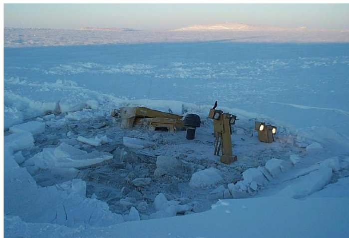
Figure 3: Breakthrough of a D10 Caterpillar tractor following formation of a circumferential crack pattern
